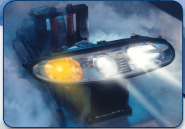
Headlamp in combined thermal cycling/vibration testing.
