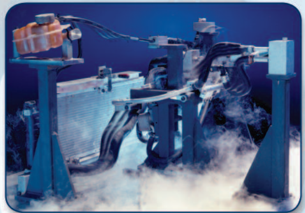
Coolant/heater hoses in combined pressure/vibration/temperature testing.
