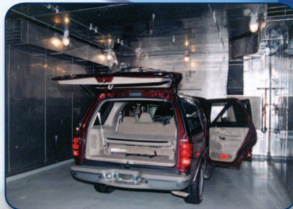
The NTS drive-in thermal chamber is 5,000 cubic feet, -40° to +100° centigrade.
